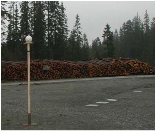
Fig. 4 Height of burst test, HOB = 2 m, using the HE C-4. Along the ground 4 sensor platforms are positioned at increasing distances of d = 4, 5, 6 and 10 m
