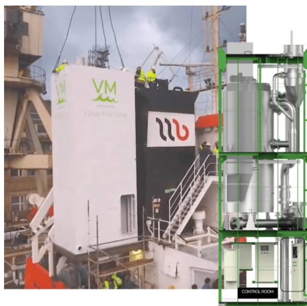
Figure 22. RAD technology incorporated in \text{SO}_2 scrubbing installations of Value Maritime to filter exhaust gases of seagoing ships.
