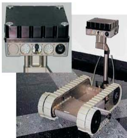
Fig. 15. REDOWL system mounted on PackBot tactical mobile robot
