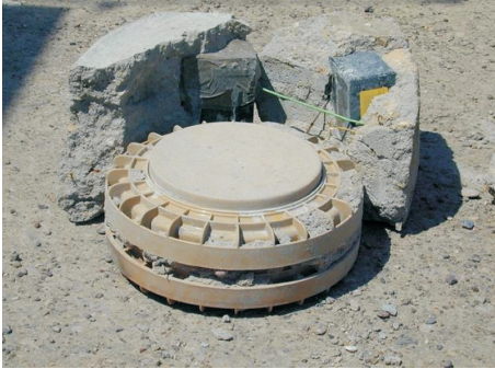
Fig. 1 Anti-Tank mine encased in concrete and command detonated via remote control [2]
